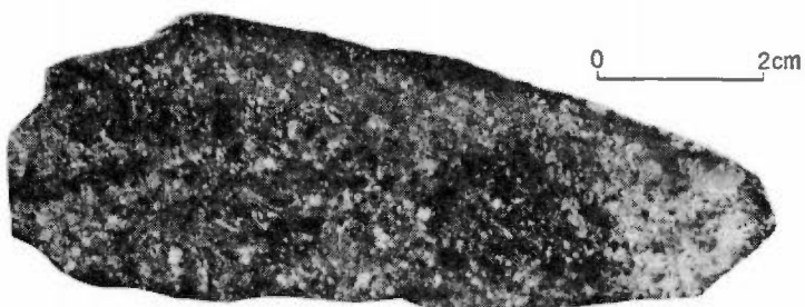
1. 流紋岩質凝灰岩の外観、もっとも石英斑岩様の部分 (6506-27, 篠河) Polished surface of rhyolitic (welded) tuff of the most "quartz porphyry" looking specimen.
