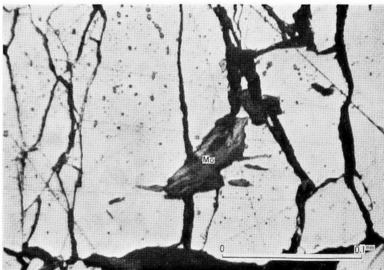
Plate 19 Cracked pyrite filled with carbonates. Molybdenite (Mo) shows a replaced figure, and it is not cut by the carbonates veinlets (SI-230, Main Tunnel, G 243+20.5').
