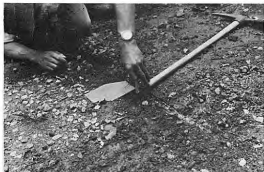
1. Ground cracks near loc. I-3 reflecting the earthquake faulting.
