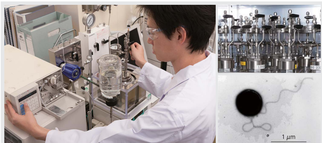
Left: High-pressure culture system. Upper Right: Vessels for simulating subsurface conditions. Lower Right: A newly isolated methanogen.
