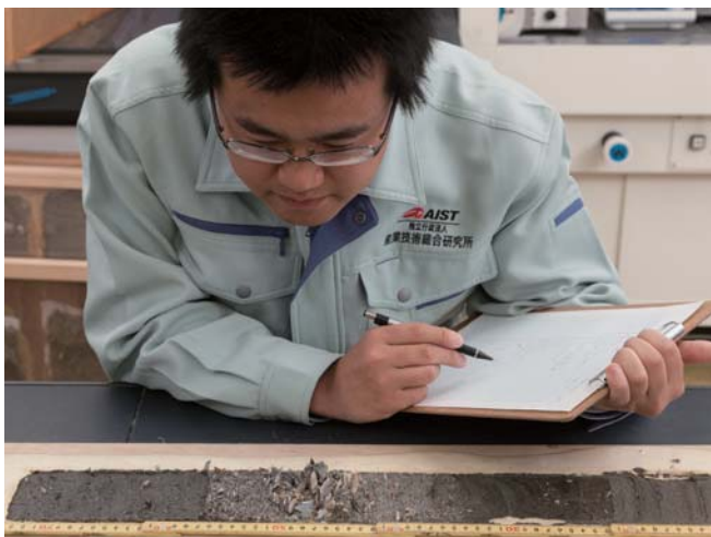
Left: Looking for lithofacies in a core sample obtained from Hirota Bay, Iwate Prefecture. Right: Numerical simulation of the AD 869 Jogan earthquake tsunami, northeastern Japan.
