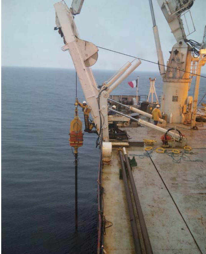
Left: Long piston coring during methane hydrate exploration in the Sea of Japan. Sedimentary cores up to 40 meters long were recovered. Right: Results of a submarine topography survey using multibeam echo sounders (MBESs). This Figure shows seabed-surface information and the echo sound record around an area of submarine hydrothermal resources.
