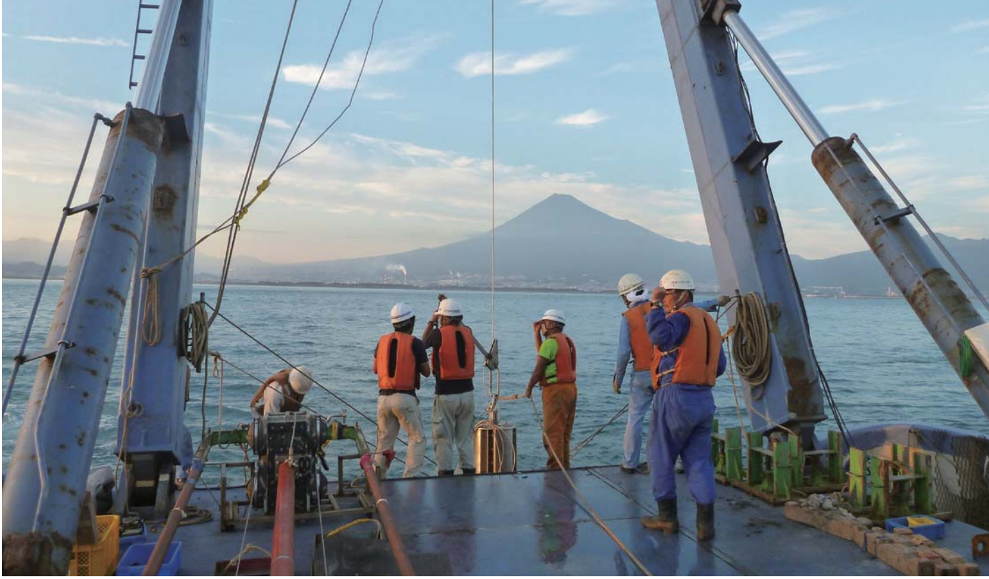
Piston-coring survey in Suruga Bay. By such surveys we aim to determine the sources of large-scale earthquakes; obtain seamless data on active faults on land and sea; determine the structure of alluvial layers; and map geological, geophysical, and active structures.
