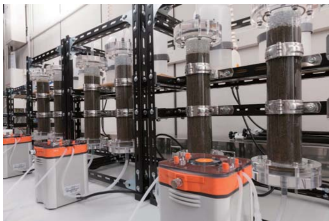
Left: Column testing systems for characterizing the leaching and transport properties of contaminants in soils.
