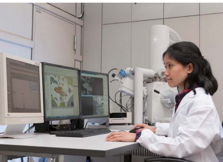
Left: Mineral Liberation Analyzer. The system is used to analyze ores by using an electron microscope with an energy dispersive spectrometer. It rapidly calculates statistic data, such as the species and grain size of constituent minerals. Right: Exploration drilling in South Africa. The drilling is assessing the grade and distribution of a newly found heavy rare-earth deposit.
