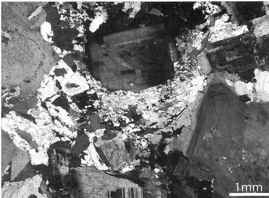
Fig. 17. Mylonitic texture in the Takidani Pluton.
