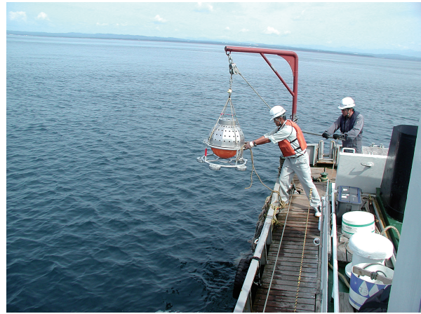
写真1 海底重力調査。 Photo.1 Measurement of sea floor gravity.
