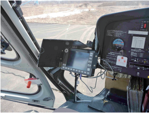
第 4 図 機上ナビゲーション装置。 AGNAV 社 PNAV-2100。進入・離脱点の入力や航跡の表示などを行い、調査飛行中はナビゲータが操作する。 Fig.4 Airborne navigation system. PNAV-2100 by AGNAV, Canada. This equipment is used as inputs of waypoints and displays of flightline paths and operated by a navigator during the survey.
