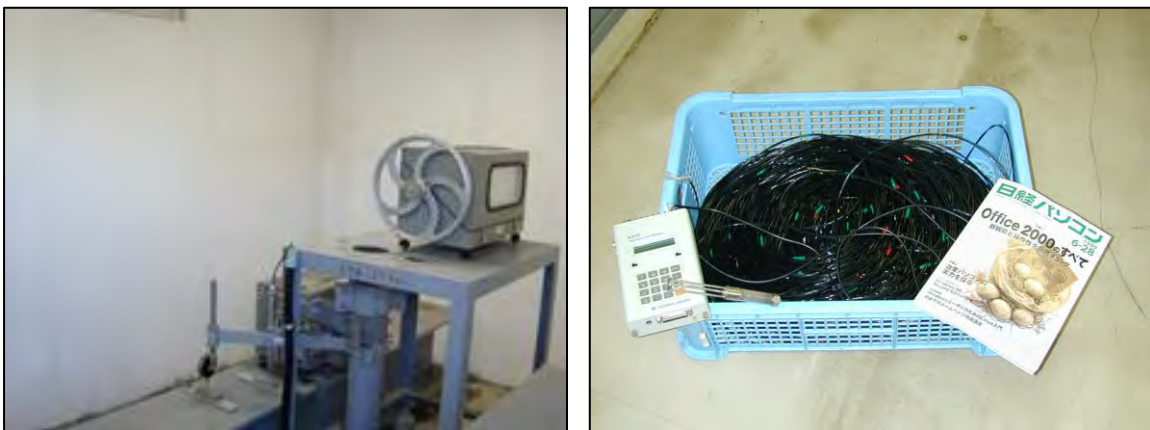
Photo 1. Observation well for monitoring of groundwater level and land subsidence in Japan (left), digital thermistor with 300m cables (right), respectively.
