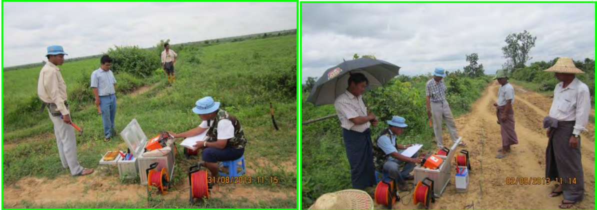
Fig. 6. Surface Geophysical Surveying using SAS 1000 Terrameter
