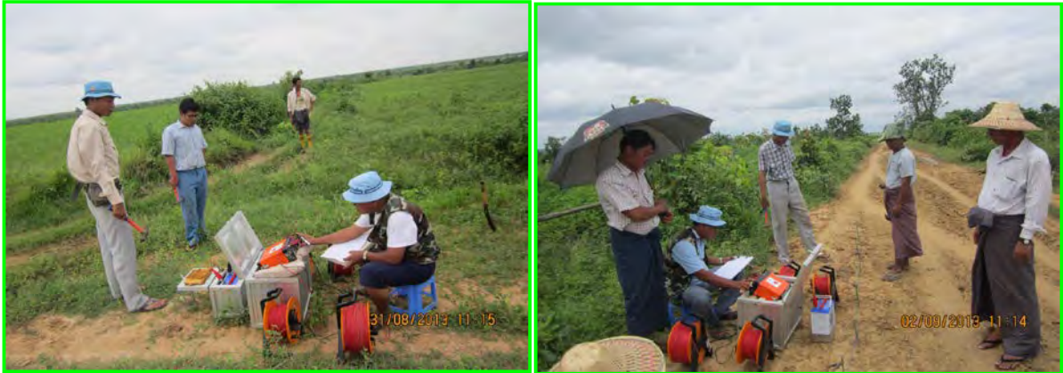
Fig. 6. Surface Geophysical Surveying using SAS 1000 Terrameter
