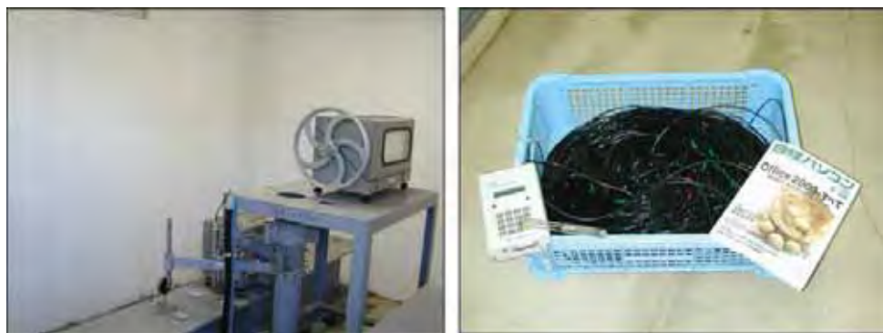
Fig.4. Observation well for groundwater level and land subsidence (left) and digital thermistor (right)
