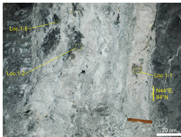
Fig. 3 A working face of the Shosen No. 2 vein at 10 ML, E45B looking towards the northeast (Loc. 1 in Fig. 2). Dotted circles on the vein indicate the area of druses where stibnite samples for sulfur isotopic measurements were collected. Loc. 1-1, Loc. 1-2 and Loc. 1-5 indicate the sample names that correspond to those in Table 1.
