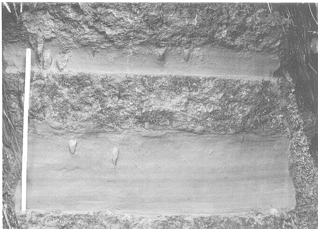
Fig.6 Alternation of turbidite sandstone and sandy mudstone in the upper Kawaguchi formation in the western part of the study area. Locality is at 1b in Fig.10.
