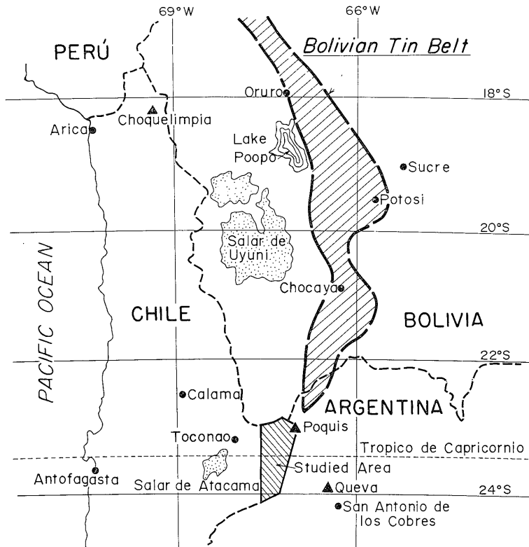
Fig.2 Bolivian tin belt (shaded area) and polymetallic Ag-Pb-Sn-Sb-Cu mineralizations (triangles) occurring to the south. After GRANT et al. (1976).
