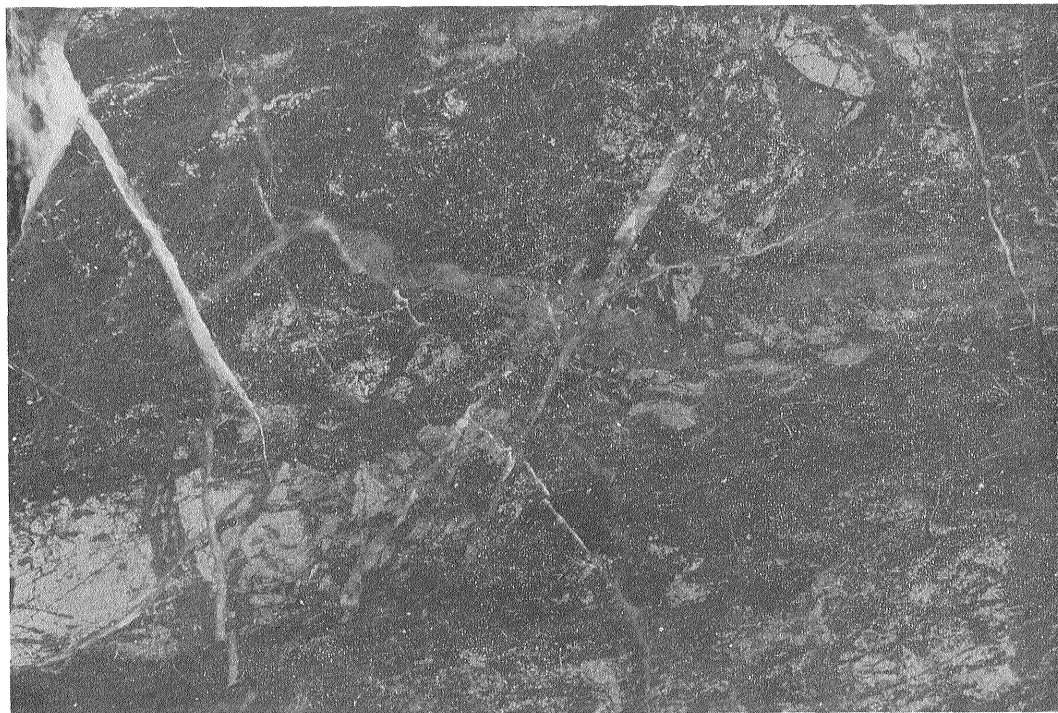
2. Limestone, blackish grey, composed of micrite incompletely soaked in black discolouration. Several sets of white calcite fracture fillings offset each other. (Sample No. 27-10, from Hanezuru Mine) \times 2.6
