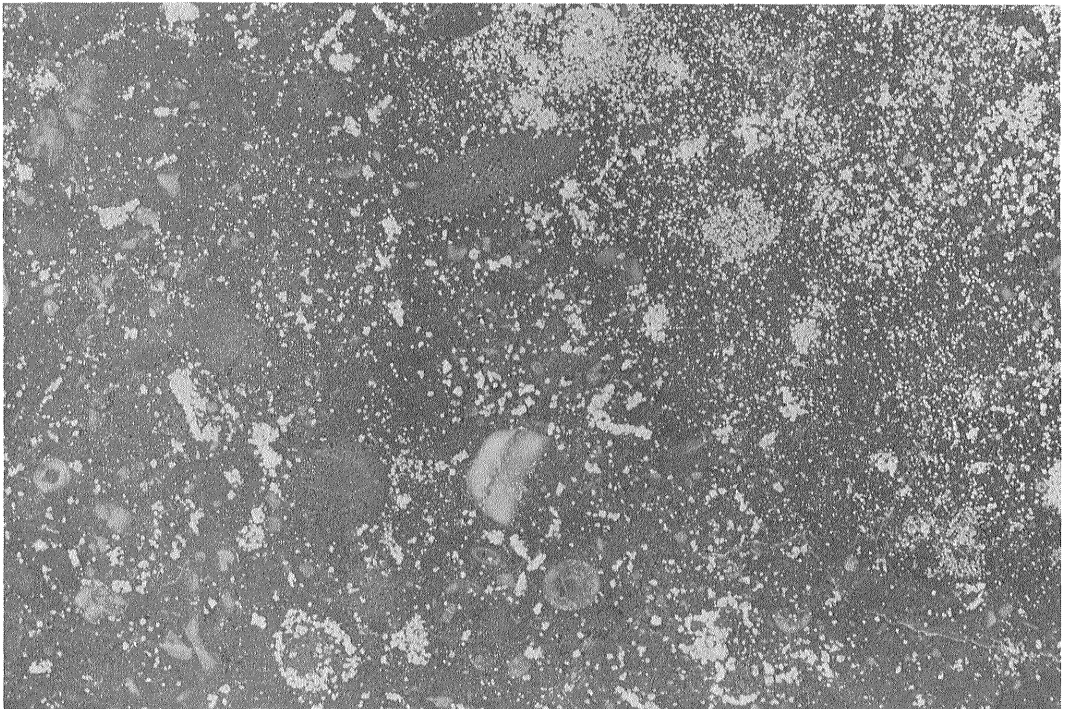
2. Lower Black Limestone, blackish grey, composed of coarse crinoid and fusulinid fragments in a black matrix. Dolomite crystals in clusters disseminated throughout the matrix (Sample No. 23-07, from Izuru) \times 2.6
