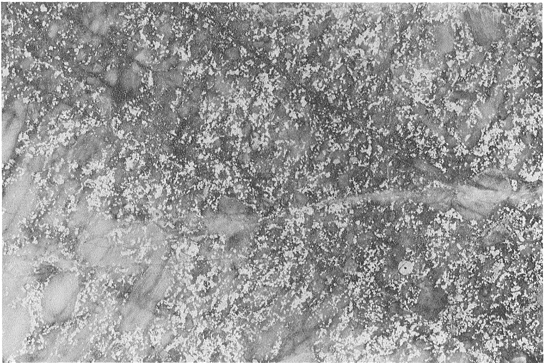
1. Upper Light-coloured Limestone, brownish grey, composed of coarse crinoid and fusulinid fragments, with finely disseminated dolomite crystals in the matrix. Black carbonaceous material in stringers and as coating of dolomite crystals (Sample No. 612-06, from the Hanezuru Mine) \times 2.6
