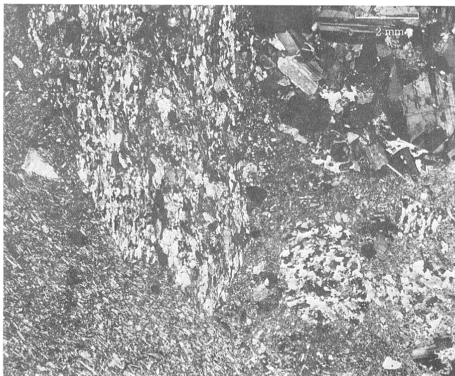
Figure 13 Photomicrograph of Kamochi conglomerate (Photomicrographs of Figs. 8~13 by Y.MASAI)
