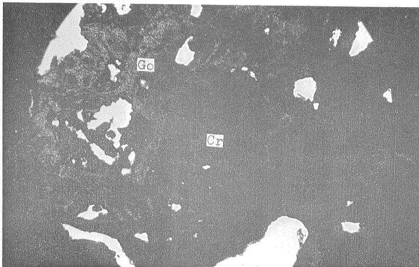
Plate 5 Chromite Cr and goethite Go in laterite. Plane polarized light. \times 200
