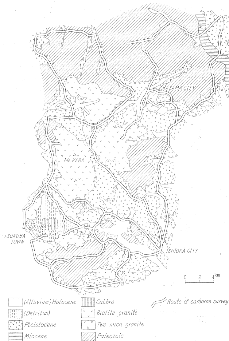
Fig. 2 Geology of the surveyed area
