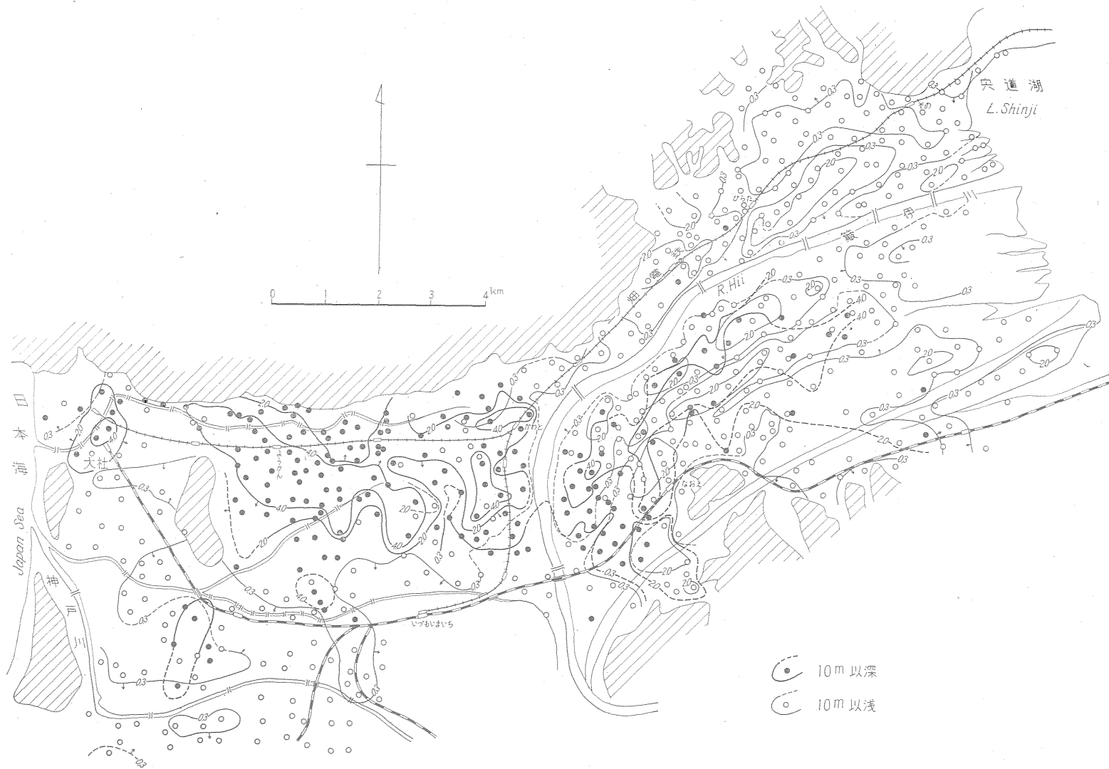
第9圖 水中溶存メタン Map showing the distribution of dissolved CH 4 (cc/l=% of meter x 6) of underground water in the Hikawa plain, Shimane Pref.
