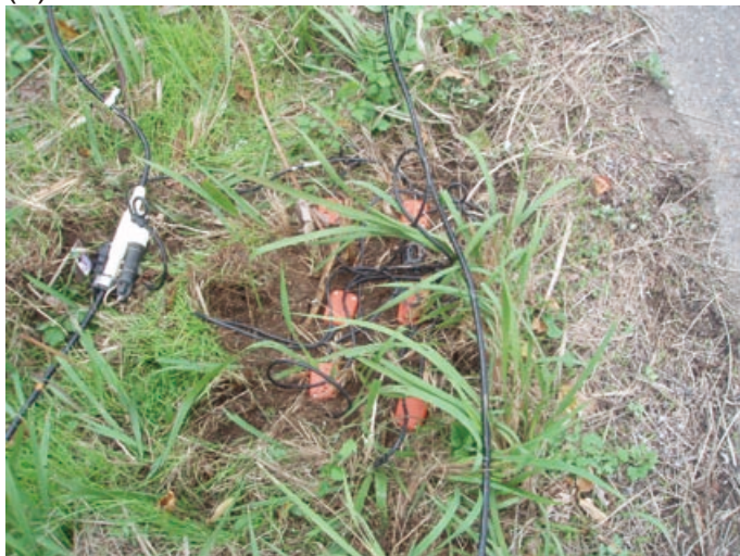
第3図. 調査機器. (a) 震源装置 (MiniVib), (b) 受振器の設置状況. Fig. 3. Survey equipments. (a) Seismic source (MiniVib). (b) Receiver array.
