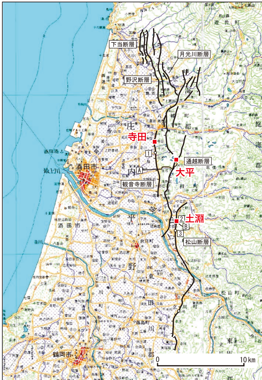
第1図. 庄内平野東縁断層帯の分布および調査地点. 断層分布は推本, 2002に基づく. 基図は国土地理院発行数値地図 200,000 分の1「酒田」「新庄」を使用. Fig. 1. Distribution of Shonai-heiya-toen fault zone and locations of paleoseismic trenches. Detail fault distribution is based on HERP (2002). Topographic base maps are from 1:200,000 Sakata and Shinjo published by Geographical Survey Institute.
