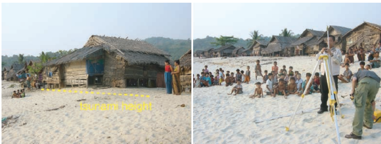
Photo 5. Survey at Sann Lan Village. Yellow dotted line is tsunami height (left). Measurement at Sann Lan Village (right).
