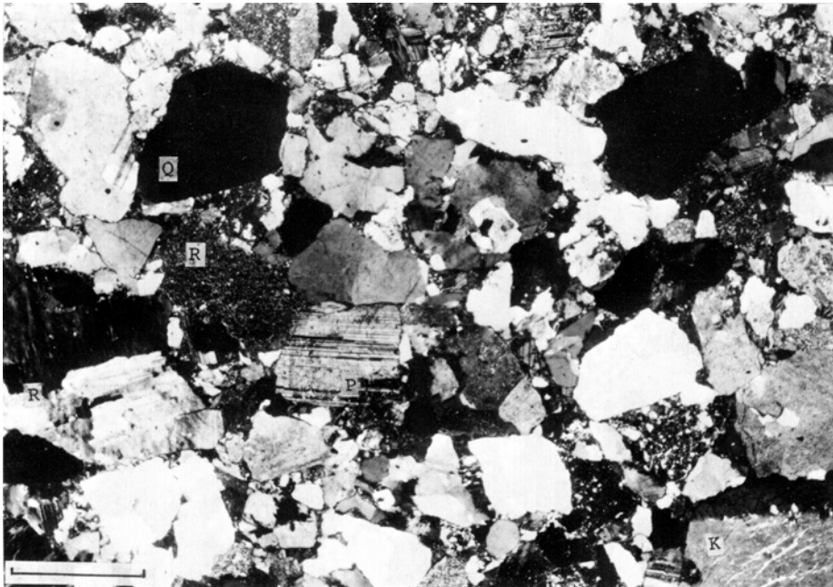
2 音無川層群羽六累層上部層の砂岩顕微鏡写真(Q:石英, P:斜長石, K:カリ長石, R:岩片, 直交ニコル, スケールは1mm) Microphotograph of sandstone in the Upper member of the Haroku Formation in the Otonashigawa Group (crossed nicols) (Q: Quartz, P: Plagioclase, R: rock fragments. scale: 1 mm)
