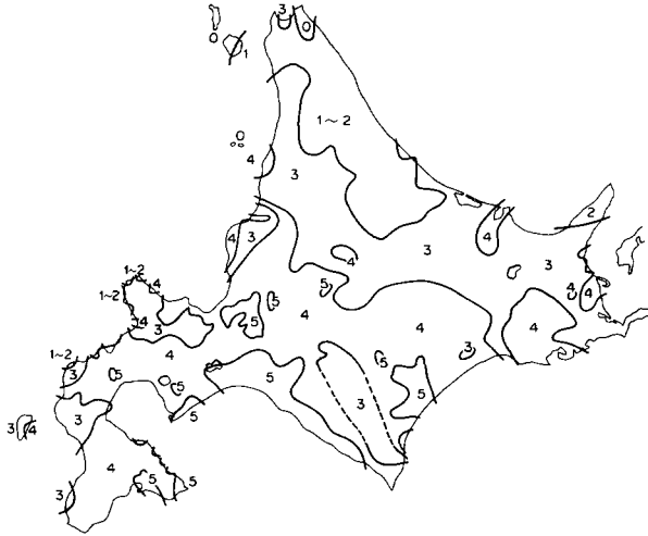
第59図 1968年十勝沖地震の震度分布図 Distribution of seismic intensities of Tokachi-oki Earthquake, 1968, after Dep. Geoph. Fac. Sci. Hokkaido Univ. (1969)
